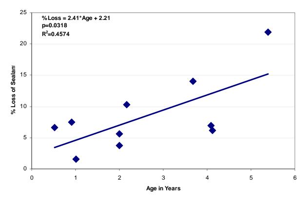
Figure 7. Linear relationship between sealant loss and age of sealant.
