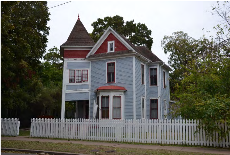
Fig. 4-1-13. This house at 909 W. 22 ½ Street is an excellent example of the irregular plan . Constructed in 1910, it has a complex roofline consisting of gables and hipped roofs, as well as an angled turret. This form was often used in association with the Queen Anne style, including differing wall textures, wood shingles, decorative door and window surrounds, and bay windows. Source: Photo by HHM, 2019.
