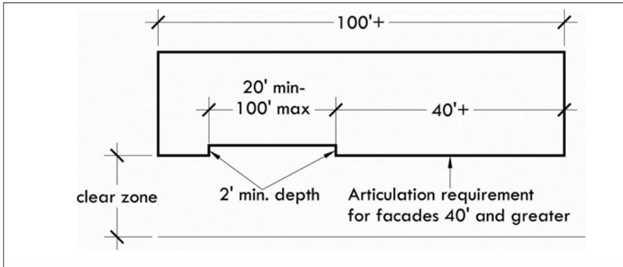
**Figure 5-4:** Illustration showing building façade articulation requirements
