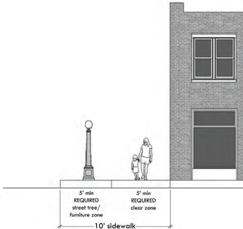
**Figure 3-16:** TOD Local Street sidewalk width requirements
