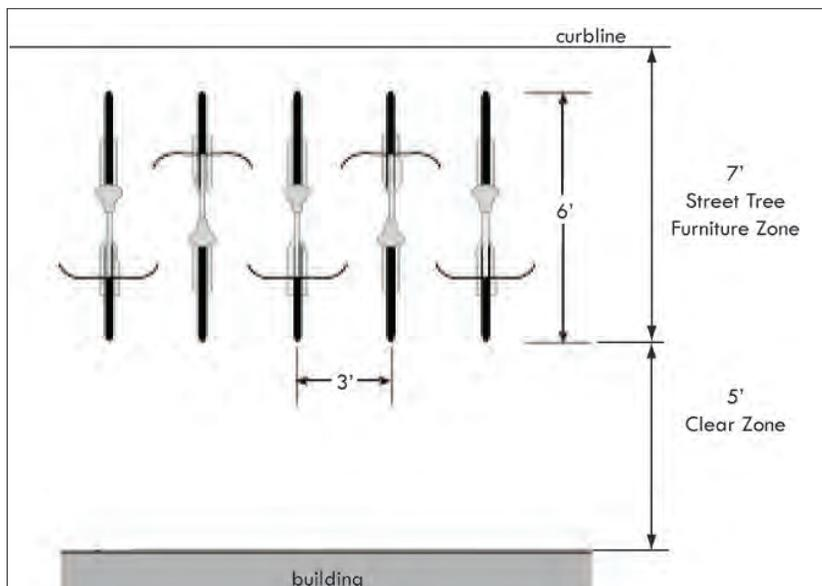
**Figure 4-15:** Bicycle parking design – Pedestrian Priority Street sidewalk
