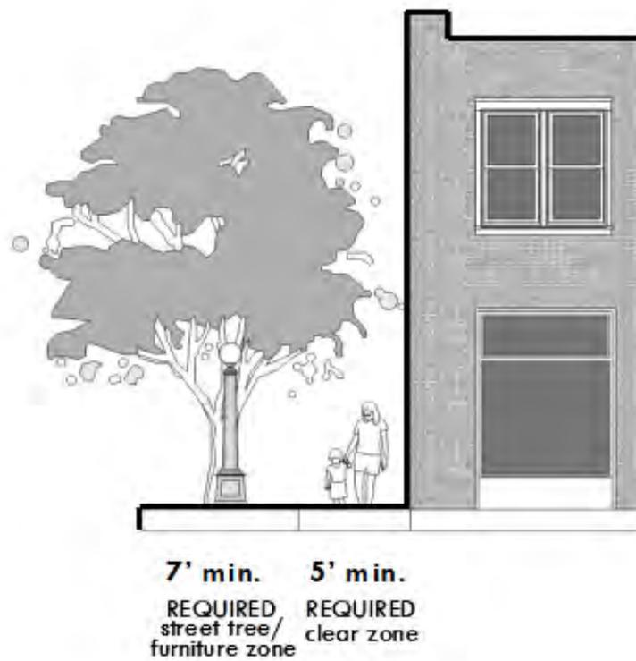
Figure 3-12: TOD Pedestrian Priority Street sidewalk width requirements.
